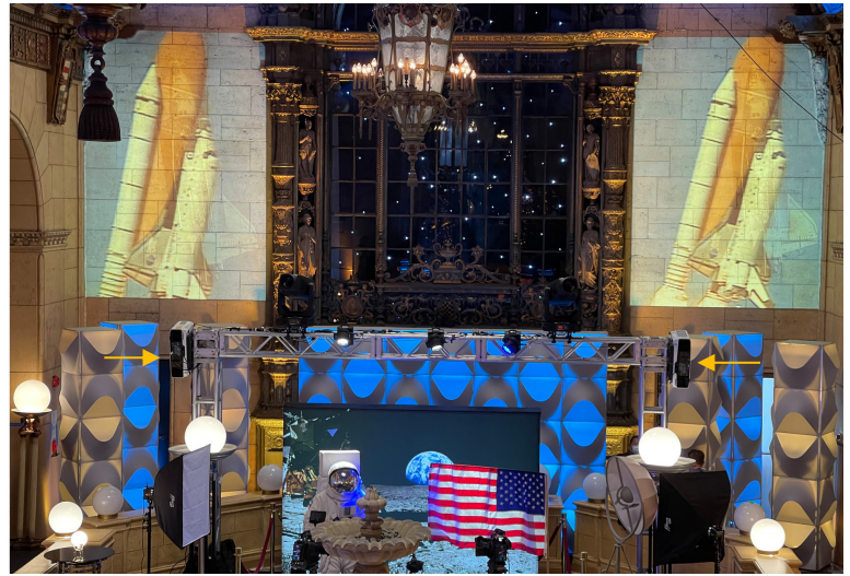
Epson's Pro L 1750UNL 15,000-lumen projectors, mounted sideways on truss and MadMapper software pixel maps for precise placement
