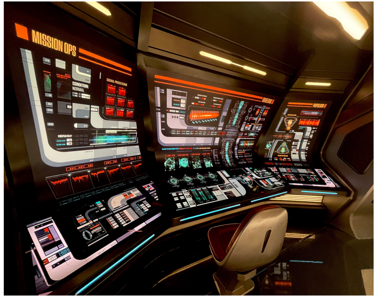
At right: Epson's projectors' dynamic imagery lit up Screen Innovations' Flex Glass curved rear-projection screens, which melded with OLED displays to create the stunning curved consoles onboard the ship. Left: Behind the screens, Epson's projectors illuminate the complex curves of the wrap-around console screens
